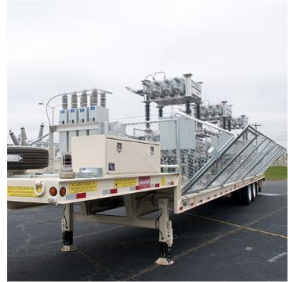
Mobile Capacitor Banks
