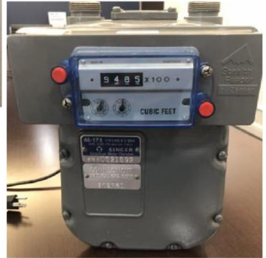
Figure 13: Gas Meter with MIU installed
